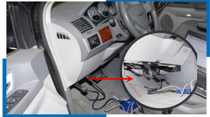
EDR download through the diagnostic link connector (DLC)
